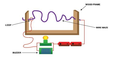
Figure 42: Model of a circuit that shows how electrical energy (generated by batteries) can control movement
