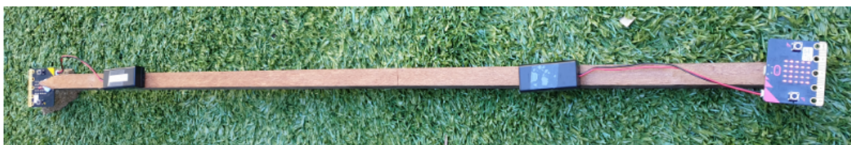
Figure 13: A micro:bit metal detector made with two micro:bits, two battery packs and a wooden garden stake
