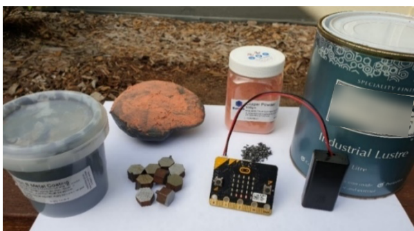
Figure 2 shows items that do not work with the micro:bit. L–R, clockwise: A metal coating paint, a rock with most of these materials on it (which the micro:bit cannot detect), copper powder, metal filings, paint with micaceous iron oxide in it and a handful of metal pieces.
