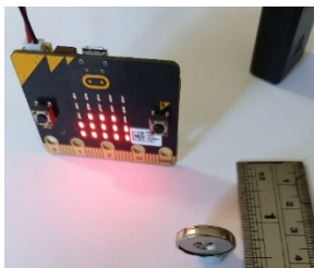
Figure 4: micro:bit detection of the sewable magnet at various distances
