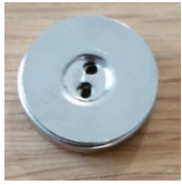
Figure 3: A sewable magnet
