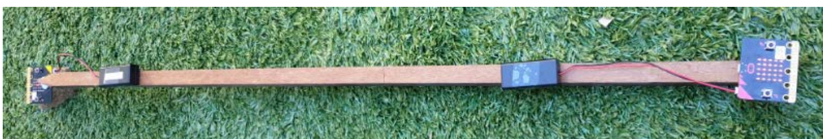
Figure 13: A micro:bit metal detector made with two micro:bits, two battery packs and a wooden garden stake
