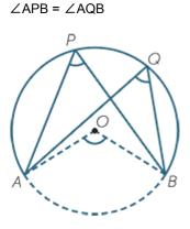
In the diagram, the two angles  $\angle APB$  and  $\angle AQB$  are subtended by the same arc AB.
